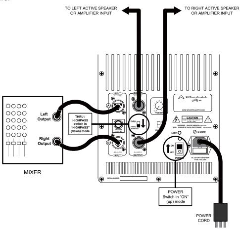
NOTE: This same connection configuration can be used with OUTPUT A and B used in a full-range mode when the THRU/HIGHPASS switch is in the "THRU" (up) position.
